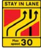
One lane crossover at contraflow road works
