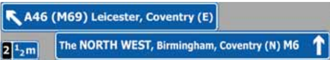
The panel with the inclined arrow indicates the destinations which can be reached by leaving the motorway at the next junction
