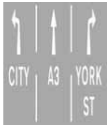
Indication of traffic lanes
