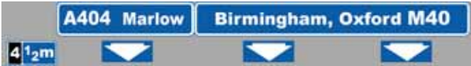
Downward pointing arrows mean 'Get in lane'. The left hand lane leads to a different destination from the other lanes
