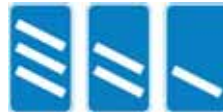
'Countdown' markers at exit from motorway each bar represents 100 yards to the exit). Green-backed markers may be used on primary routes and white-backed markers with black bars on other routes. At approaches to concealed level crossings white-backed markers with red bars may be used. Although these will be erected at equal distances the bars do not represent 100 yard intervals.
